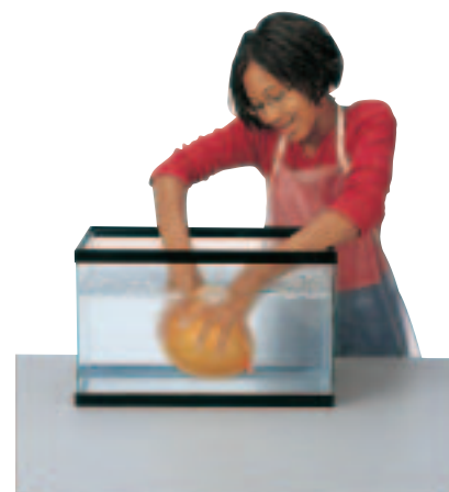
Figure 23 Charles's law states that as the temperature of a gas is lowered, the volume decreases.
