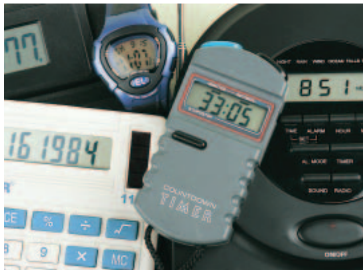
Figure 12 Liquid crystals are used in the displays of watches, clocks, calculators, and some notebook computers because they respond to electric fields.
